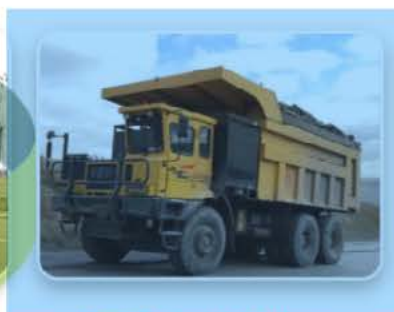
B-S Electric Mining Truck (70 tons)
