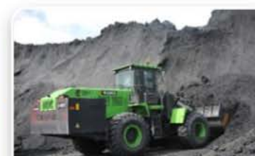
Electric Loader (5.5 tons)
