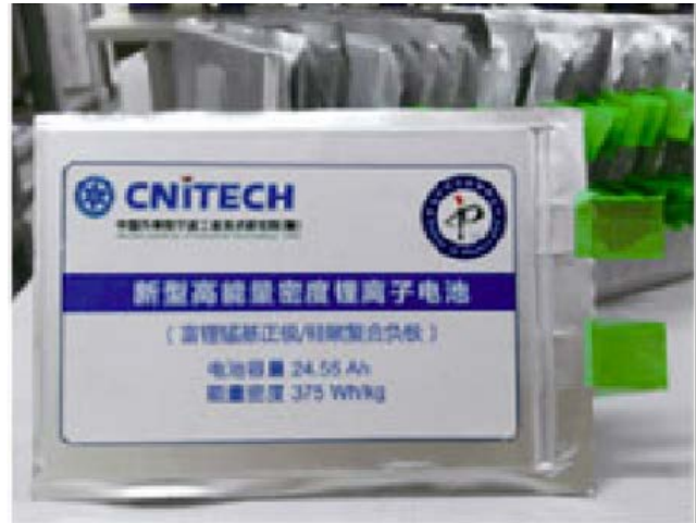
Figure 6: High energy density Li-ion batteries using Li-rich layered cathode
