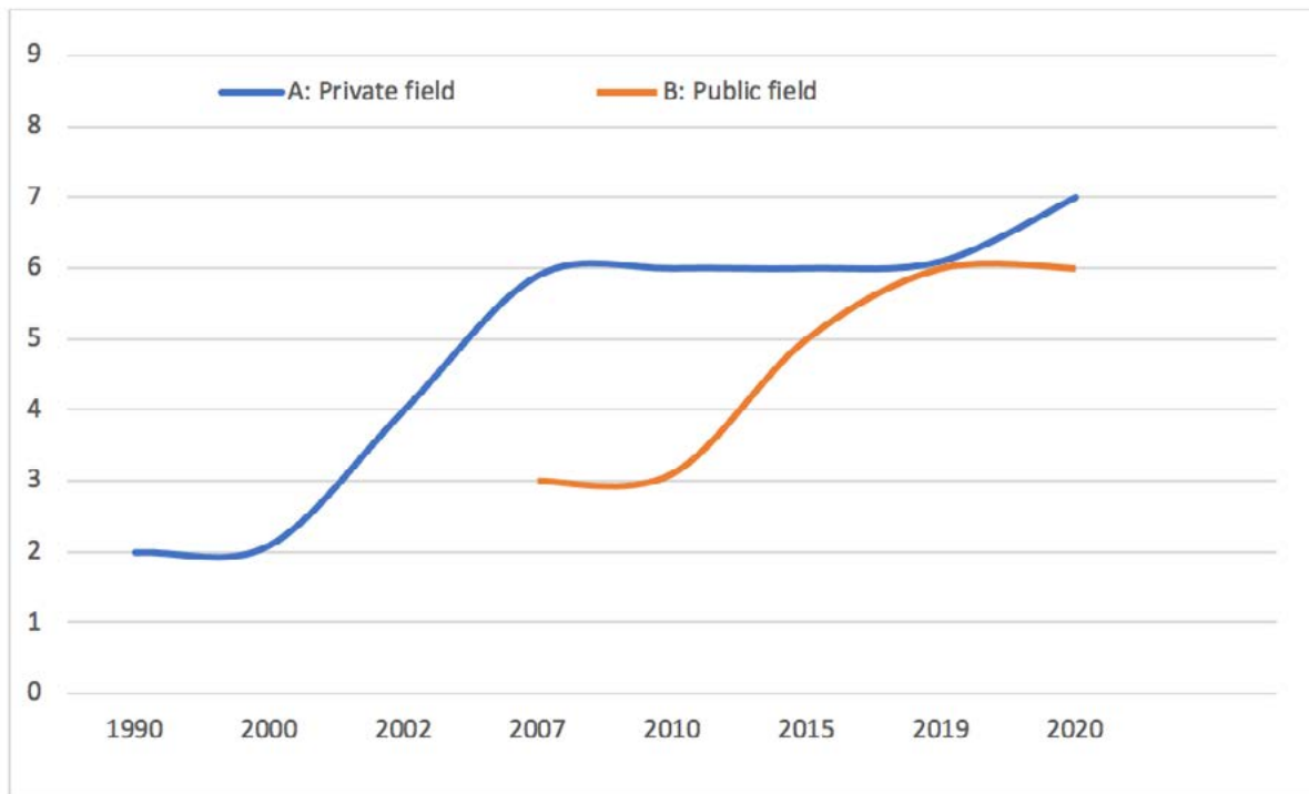
Figure 5: TRL development of China's EV WPT technology Edited and drawn by Shengdong Zu
