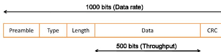
The figure shows an example where the physical wireless link enables 1000 bits/second but where the actual information transferred is 500 bits/second (the data in the packet shown).
