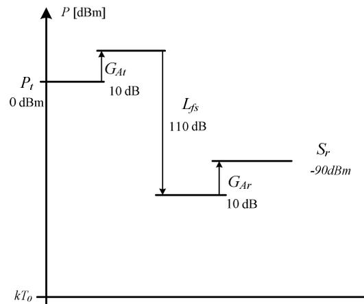
The figure shows the link budget diagram for BS1. The base station needs 0 dBm to be able to communicate with the base stations (BS2) which have a sensitivity of -90 dBm.
