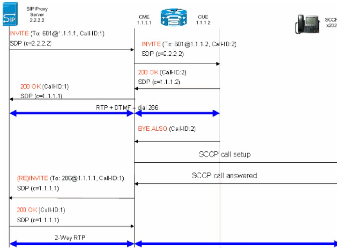
If REFER is supported on the SIP proxy, the user portion of the Refer-To and Referred-By must be translated to a DID that the SP proxy understands. The host portion of the Refer-To and Referred-By fields must be an IP address or DNS that the SP proxy can route to as well (this occurs by default on CME 4.1).
