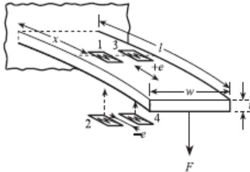
a) Four identical strain gauges (specified below) are to be bonded onto the cantilever halfway along its length as shown in above figure.
