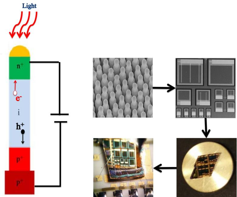
The samples were prepared by first depositing gold catalyst nanoparticles on a  $p^+$  InP substrate using an aerosol technique and subsequently growing NWs using MOVPE. The processing of the detectors include deposition of  $\text{SiO}_2$ , followed by an etching step to remove the oxide from the tip of the NWs, and finally sputtering of ITO on  $1 \times 1 \text{ mm}^2$  device areas (images on right-hand side).
