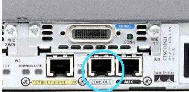
2. What kind of cable do you need to connect the console port of the router to the PC?
