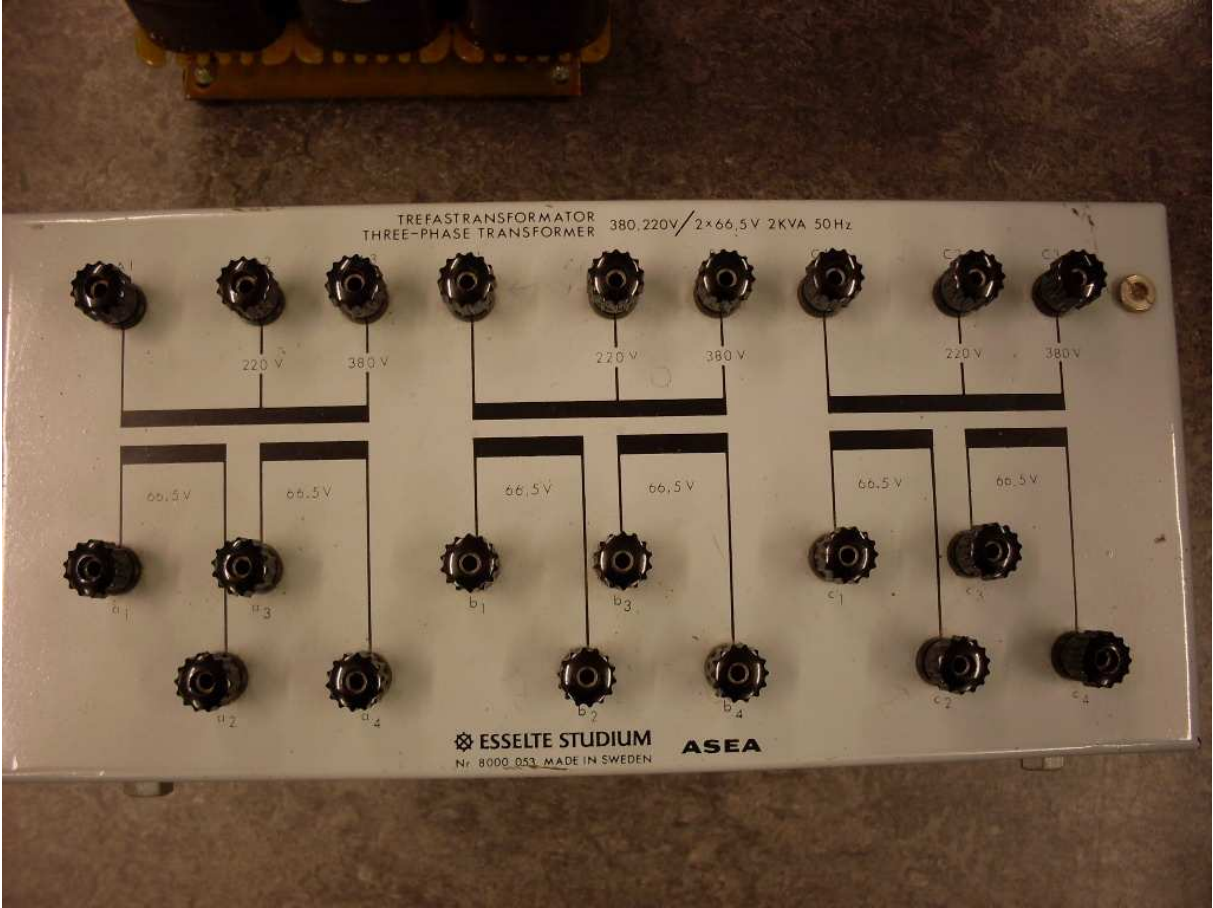
Figur: trefastransformator 2kVA
