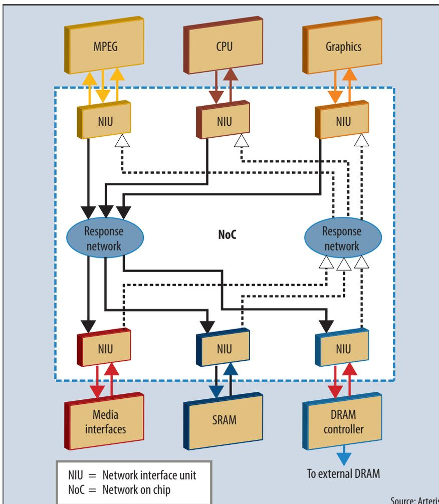
**Figure 1.** NoC systems apply networking, rather than bus, technology, to communications among the cores on a processor. Network interface units manage the packetization of native intercore data. Routers then connect the various processing cores and other elements.
