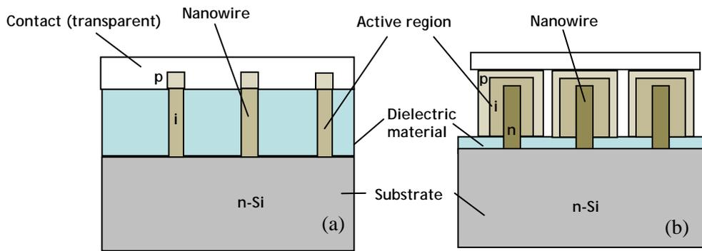
**Fig. 4** Axial (a) and radial (b) photodetector designs based on InGaAs nanowires grown on silicon
