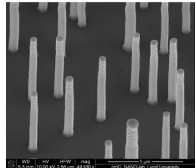
Fig. 2 SEM image of InP n<sup>+</sup>p diodes on InP.
