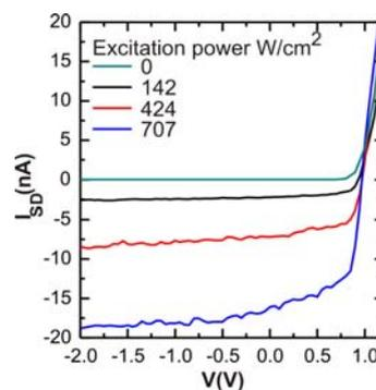
Fig. 3 I-V characteristics of InP n<sup>+</sup>p diodes
