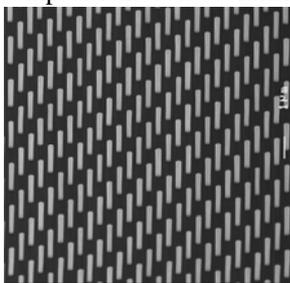
Fig. 1 SEM image of InAs NWs grown on GaAs.
