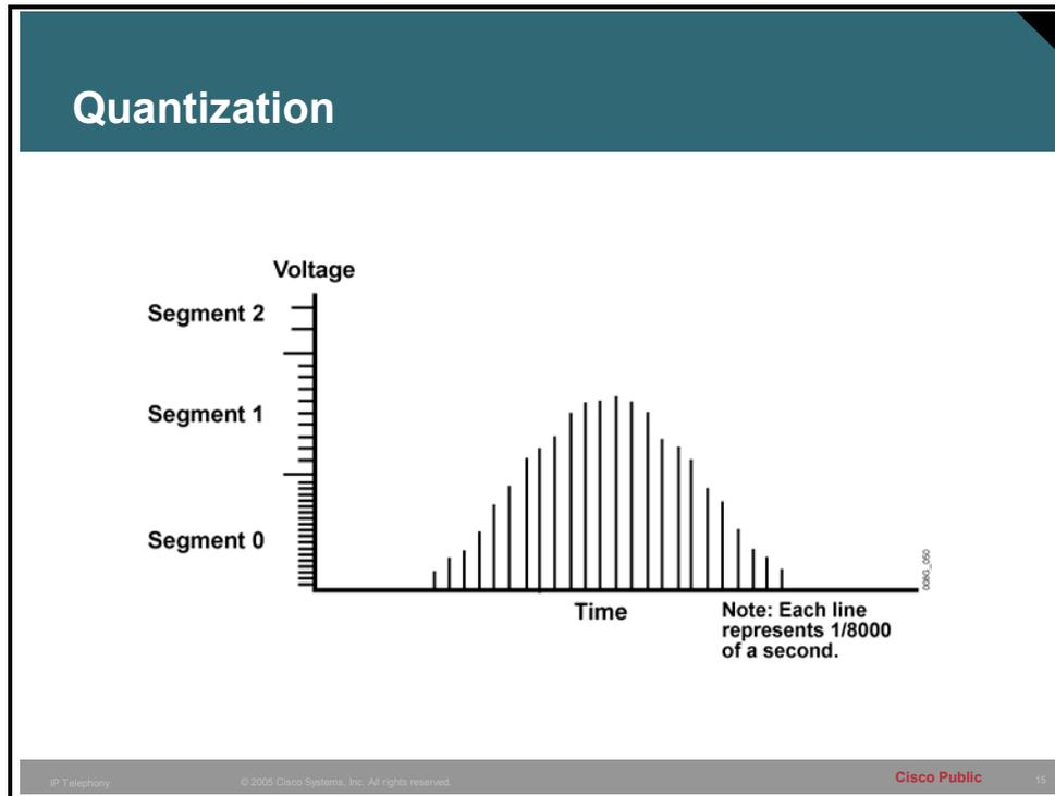
Quantization involves dividing the range of amplitude values that are present in an analog signal sample into a set of discrete steps that are closest in value to the original analog signal. Each step is assigned a unique digital code word.
