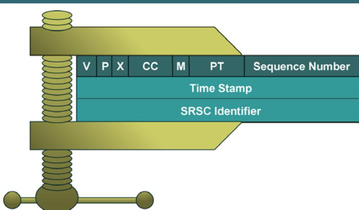
The diagram illustrates the RTP header structure and the CRTP compression mechanism. The RTP header is shown as a horizontal bar divided into several fields: V, P, X, CC, M, PT, and Sequence Number. Below these fields are two larger fields: Time Stamp and SRSC Identifier. A yellow wedge-shaped block is positioned above the header, and a spring mechanism is shown compressing the header fields. A horizontal bar with a ball end is shown below the spring, representing the compressed header.
