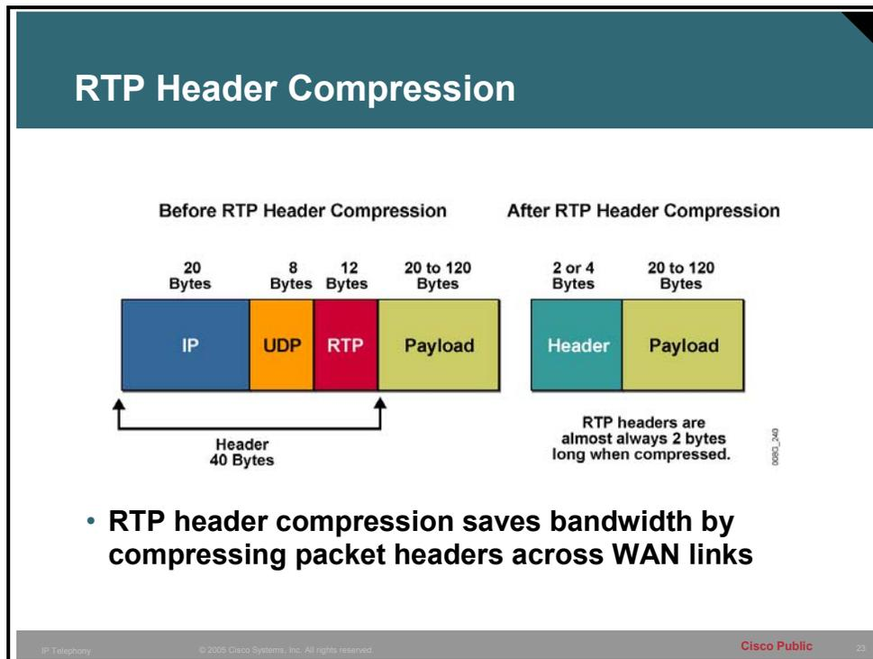
Given the number of multiple protocols that are necessary to transport voice over an IP network, the packet header can be large. You can use cRTP headers on a link-by-link basis to save bandwidth.
