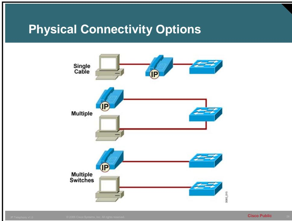
This figure depicts physical connection options for IP Phones. The IP Phone connects to the network through a Category 5 or better cable that has RJ-45 connectors. The power-enabled switch port or an external power supply provides power to an IP Phone. The IP Phone functions like other IP-capable devices sending IP packets to the IP network. Because these packets are carrying voice, you must consider both logical and physical configuration issues.
