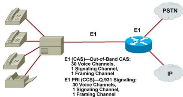
This figure depicts an E1 interface. An E1 interface has 32 channels and simultaneously carries up to 30 conversations. The other two channels are used for framing and signaling. The 32 channels are grouped to form a frame. The frames are then grouped together into multiframes (groups of 16 frames). Europe and Mexico use the E1 interface.
