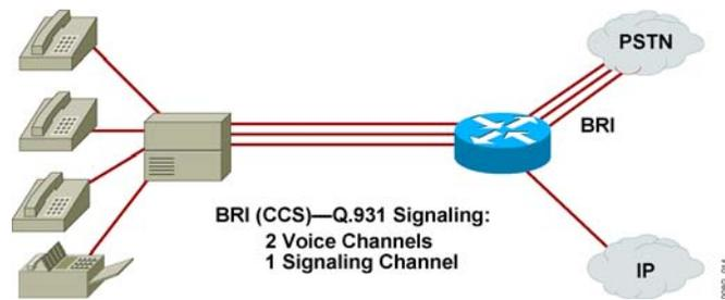
This figure depicts a Basic Rate Interface (BRI). You can use a BRI to connect the PBX voice into the network. Used primarily in Europe for PBX connectivity, BRI provides a 16-kbps D channel for signaling and two 64-kbps B channels for voice. BRI uses Q.931 signaling in the D channel for call signaling.
