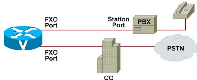
This figure depicts an FXO interface. The FXO interface allows an analog connection to be directed at the CO of a PSTN or to a station interface on a PBX. The switch recognizes the FXO interface as a telephone because the interface plugs directly into the line side of the switch. The FXO interface provides either pulse or DTMF digits for outbound dialing.
