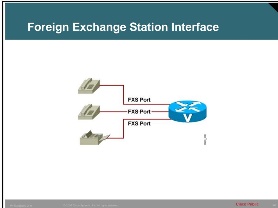
This figure depicts an FXS interface. The FXS interface provides a direct connection to an analog telephone, a fax machine, or a similar device. From a telephone perspective, the FXS interface functions like a switch; therefore, it must supply line power, ring voltage, and dial tone.
