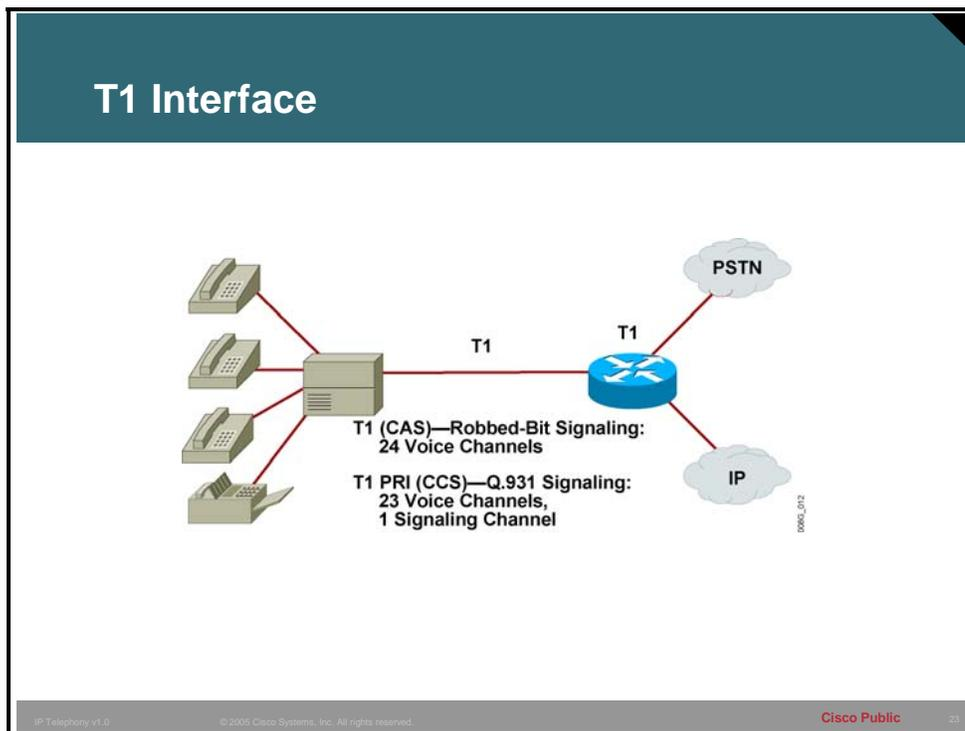
This figure depicts a T1 interface. In a corporate environment with a large volume of voice traffic, connections to the PSTN and to PBXs are primarily digital.
