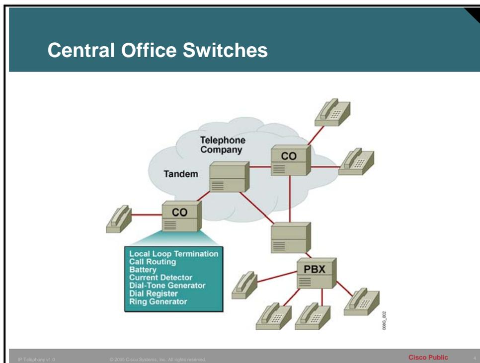
The figure shows a typical CO switch environment. The CO switch terminates the local loop and makes the initial call-routing decision.
