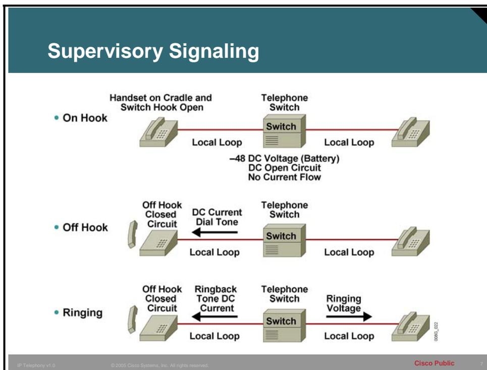
A subscriber and telephone company notify each other of call status with audible tones and an exchange of electrical current. This exchange of information is called supervisory signaling.
