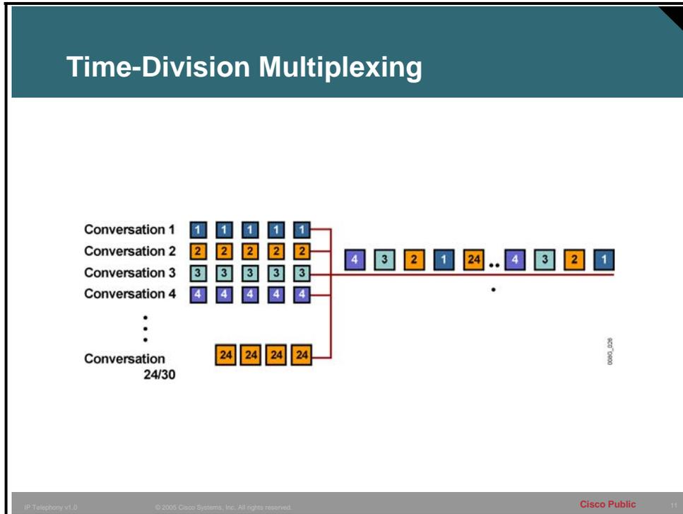
Time-division multiplexing (TDM) is used extensively in telephony networks to carry multiple conversations concurrently across a four-wire path. TDM involves simultaneously transmitting multiple separate voice signals over one communications medium by quickly interleaving pieces of each signal, one after another. Information from each data channel is allocated bandwidth based on preassigned timeslots, regardless of whether there is data to transmit.
