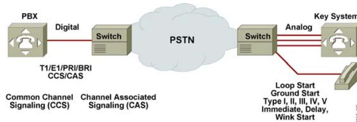
Supervisory, address, and informational signaling must be carried across both analog and digital connections. Depending on your connection to the network, you must configure specific signaling to match the type of signaling required by the service provider.
