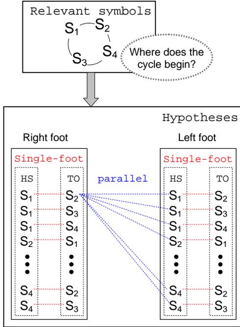
Figure 5: **Creating hypotheses.** The single step hypotheses are all pairwise combinations of the relevant symbols, and parallel hypotheses are all permutations of the right foot and left foot single step hypotheses.
