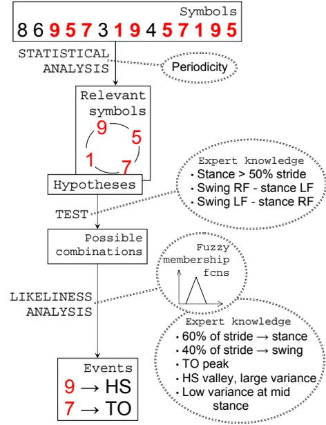
Figure 4: **Context analysis**. Graphical representation of the steps taken towards context analysis of the signal.
