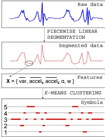
Figure 3: **Symbolization**. Graphical representation of the steps taken towards symbolization of the signal.
