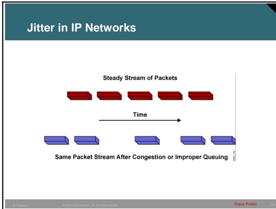
Jitter is defined as a variation in the delay of received packets. On the sending side, packets are sent in a continuous stream with the packets spaced evenly apart. Because of network congestion, improper queuing, or configuration errors, this steady stream can become lumpy, or the delay between each packet can vary instead of remaining constant, as displayed in the figure.
