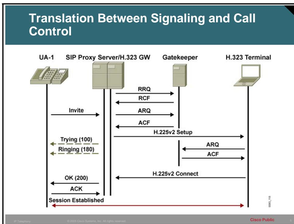
In the traditional telephone network, the individual call legs contributing to an end-to-end call often involve different signaling systems and procedures. In the graphic, an IP Phone is communicating with its SIP proxy server using the SIP protocol. However, it is also attempting to reach an H.323 endpoint. Because the two VoIP protocols are different, a translation is necessary at the SIP proxy server (namely, an H.323 gateway) to allow the two telephony endpoints to establish a connection.
