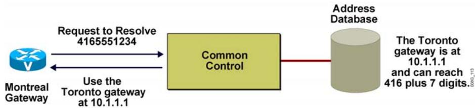
After an address is registered, it can be discovered through address resolution. Address resolution translates a multimedia user address to an IP address so that the endpoints can communicate with each other to establish a control relationship and create an audio path.
