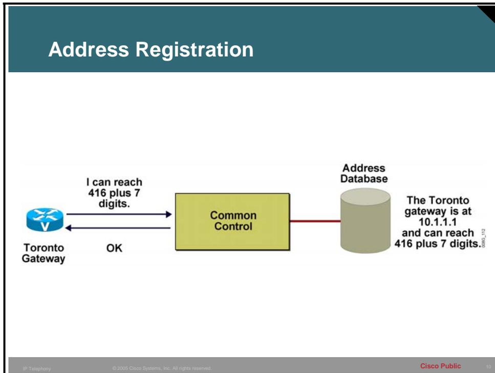
When an endpoint registers with a call control component, it supplies its telephone address or addresses and, if it is a gateway, the addresses of the destinations it can reach. The endpoint provides other information relating to its capabilities. Multiple destinations that are reachable through a gateway are usually represented by a prefix. The use of a prefix allows call control to create a database that associates a telephony-type address, for example, with its corresponding IP address.
