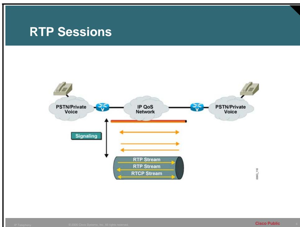
An audio path of a VoIP call leg is dependent on the creation of RTP sessions. These RTP sessions transport voice unidirectionally, so that bidirectional voice uses two RTP sessions. (In principle, if voice is needed in one direction only, as in the case of a recorded announcement or voice mail, only one RTP session is required.) The figure shows RTP sessions being created during call setup.
