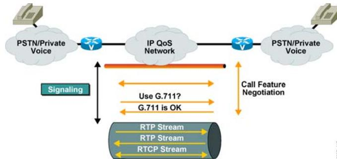
Creating the RTP sessions is not the only task of call control during call setup. The endpoints need to establish a bilateral agreement in which the communicating parties discover acceptable call parameters and then agree on the operating parameters of the call. When agreement is not possible, the call is not completed and is dropped.
