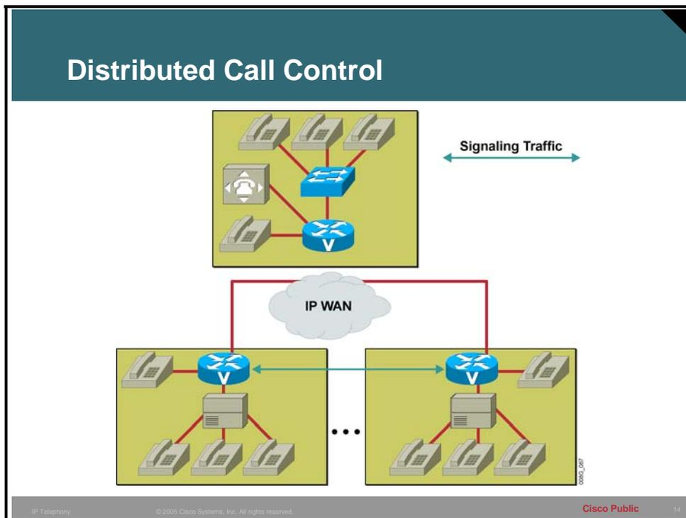
Endpoints in a distributed call control model have sufficient intelligence to autonomously manage the telephone interface and initiate VoIP call setup. Although the endpoint in a distributed model often depends on shared common control components for scalability, it possesses enough intelligence to operate independently from the common control components. If a common control component fails, an endpoint can use its own capabilities and resources to make routing or rerouting decisions.
