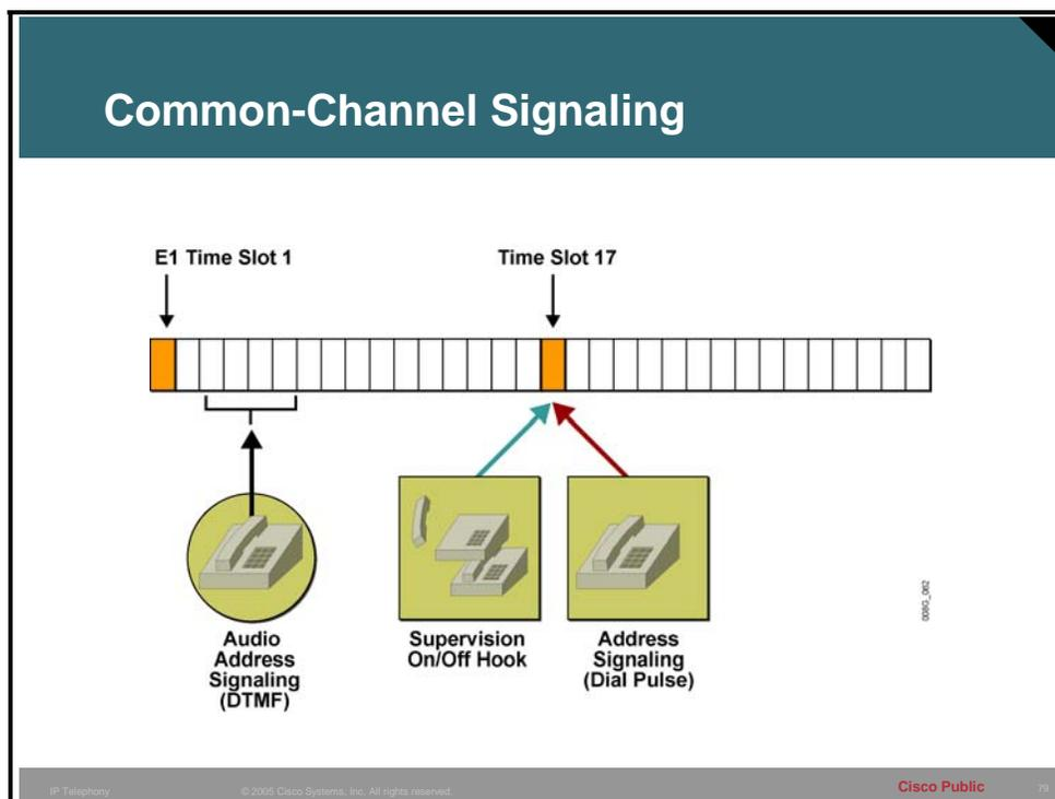
Whereas CAS uses bit time slots assigned to each specific channel, CCS uses a common channel and protocol to setup calls for all the bearer channels. Using ISDN over E1 as an example, the signaling protocol Q931 would use timeslot 17 to exchange call-setup messages for any of the 30 bearer (B) channels.
