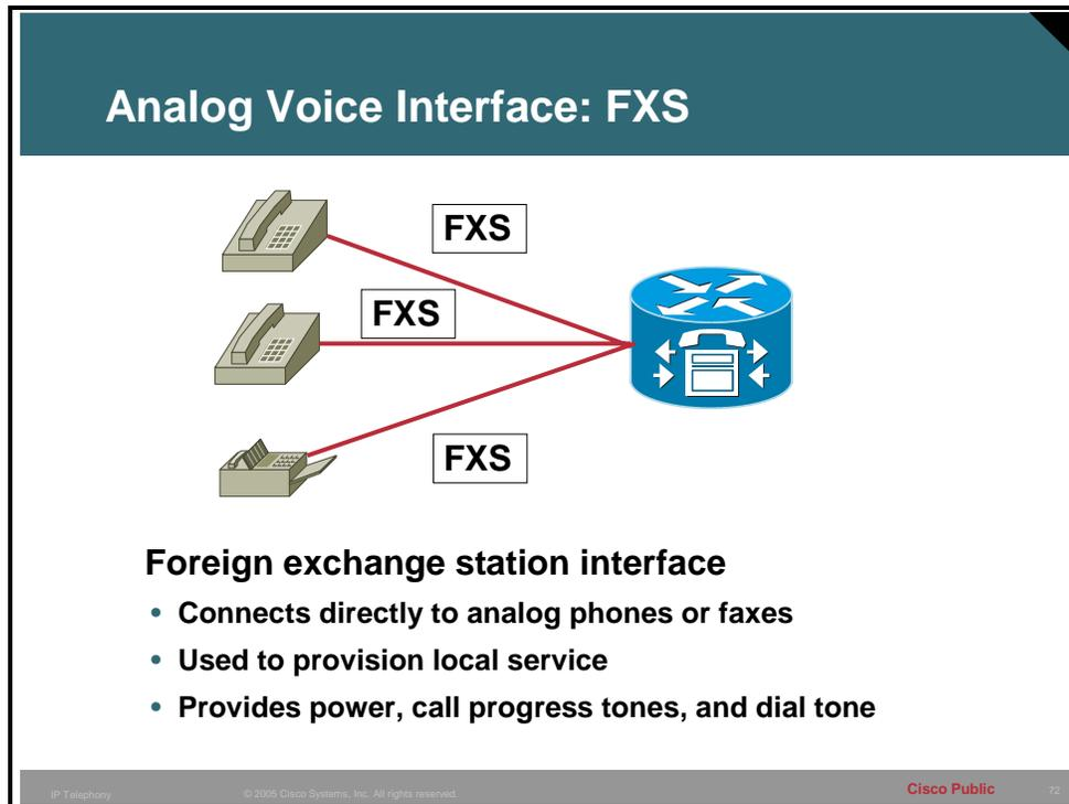
When analog phones or fax machines are used in an IP-based environment, they will need to have a connection into this IP network. This connection takes the form of an FXS interface. The FXS interface provides a direct connection to an analog telephone, a fax machine, or a similar device. From the analog device's perspective, the FXS interface functions like a switch. Therefore, it must supply line power, ring voltage, and dial tone.
