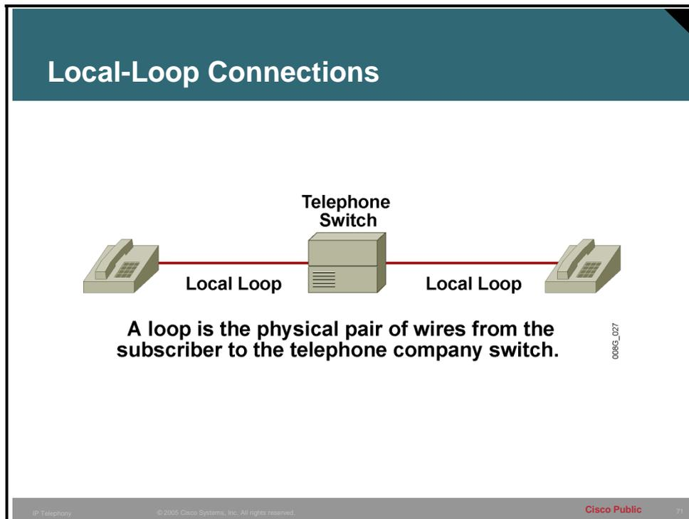
A subscriber home telephone connects to the telephone company central office (CO) via an electrical communication path called a local loop as depicted in the figure. The loop consists of a pair of twisted wires—one is called tip, the other is called ring.
