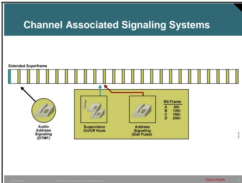
Because the signaling occurs within each DS0, it is referred to as in band. Also, because the use of these bits is exclusively reserved for signaling each respective voice channel, it is referred to as CAS.
