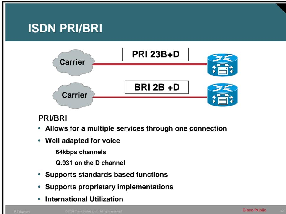
One form of Common Channel Signaling is Integrated Services Digital Network (ISDN). Primary rate interface (PRI) and basic rate interface (BRI) are the two ways of implementing ISDN.
