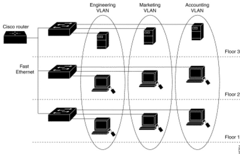
When the number of ports in a network exceeds the port capacity of the switch, you must cross-connect multiple switch chassis, which defines a trunk. The trunk is not a member of any VLAN, but a conduit over which traffic passes for one or more VLANs.
