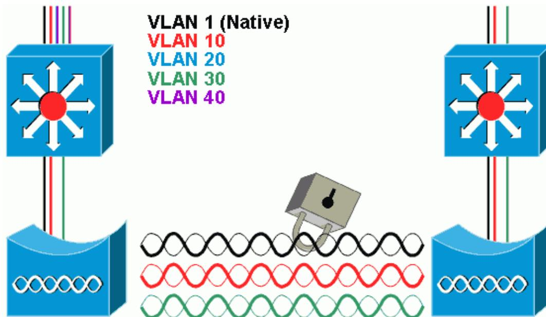
In order to encrypt data that passes over the radio link, apply encryption to only the SSID of the Native VLAN. That encryption applies to all other VLANs. When you bridge, there is no need to associate a separate SSID with each VLAN. VLAN configurations is the same on both the root and non-root bridges.
