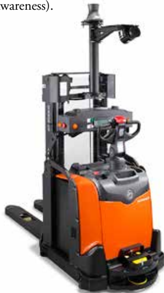
Above: A fork-lift as a part of an intelligent warehouse environment, there the fork-lift truck autonomously builds up a map of environment and do inventory of stock while working safely together with people as in the AIMS Project.
