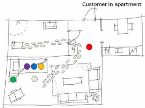
Figure 1: A wake-up scenario in a home environment equipped with several sensors. The coloured dots represent different events such as: waking up, stepping outside the bed, walking to the bathroom etc.
