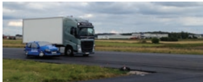
Figure 1: Balloon car being used to assess active safety systems in highway-merging scenarios.
