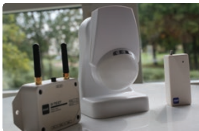
Some of the technology used in the SA3L-project. In front a transceiver, wireless IR sensor and door alarm
